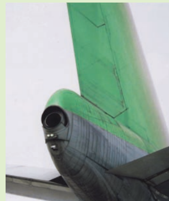
APU (Auxiliary Power Unit)
